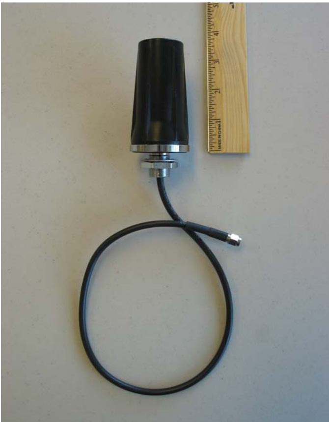
Figure VI. Dual-Band, 3dBi/5dBi, Omni, Type RM Body Mount Antenna, cable with SMA male connector
