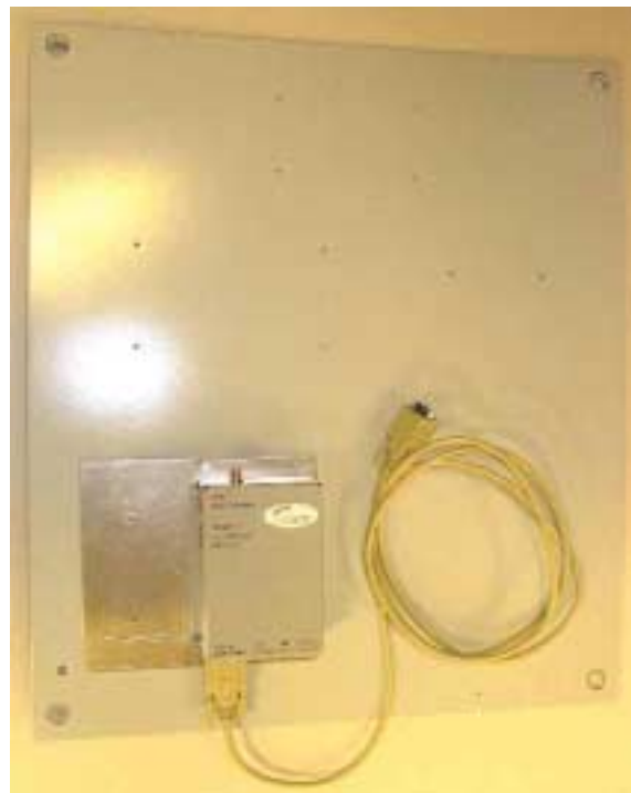
Figure 2 – RTM on PCD backplate
